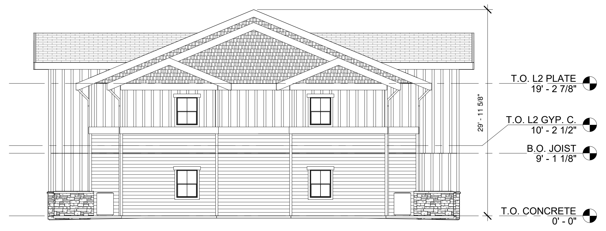
② LEFT ELEVATION - BLDG. TYPE B 1/8" = 1'-0"
