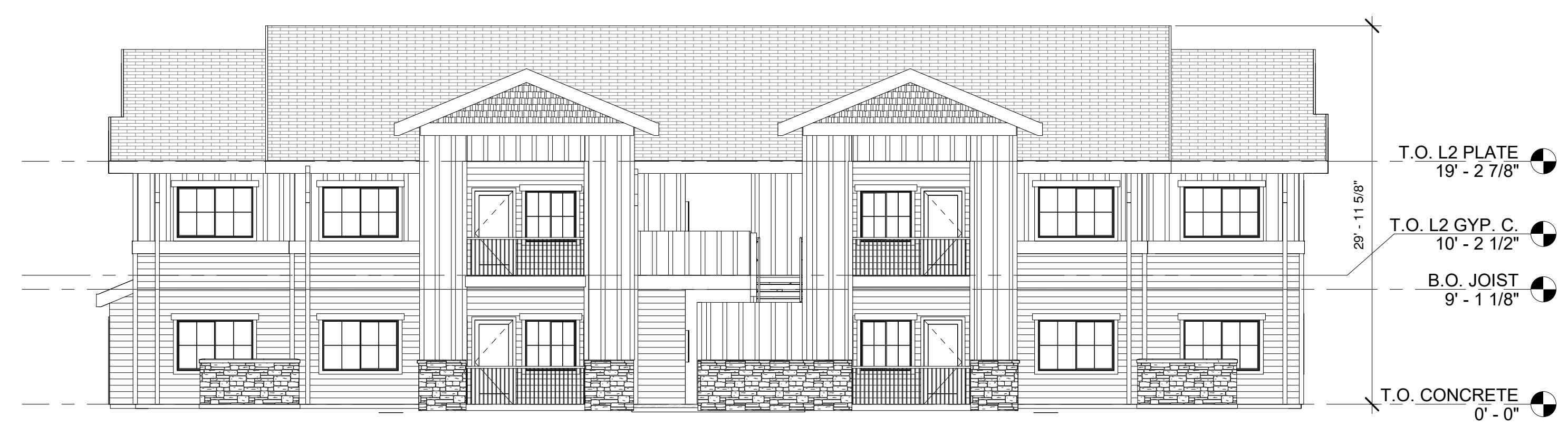
④ REAR ELEVATION - BLDG. TYPE B 1/8" = 1'-0"
