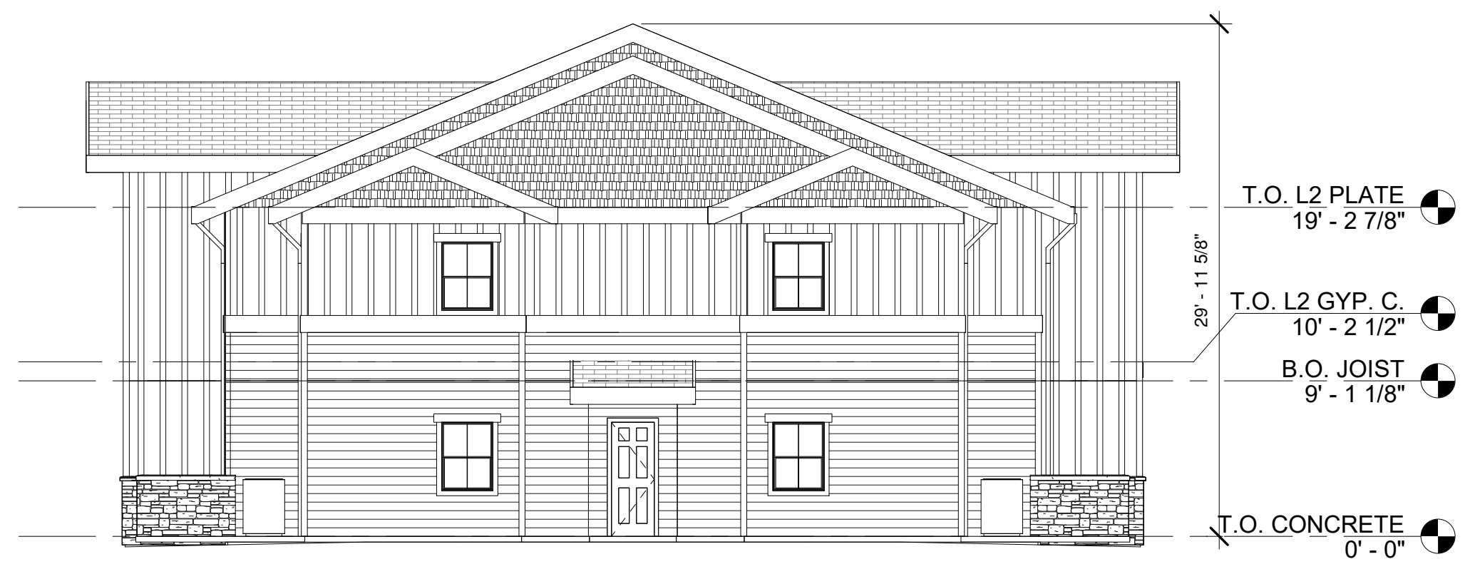
③ RIGHT ELEVATION - BLDG. TYPE B 1/8" = 1'-0"
