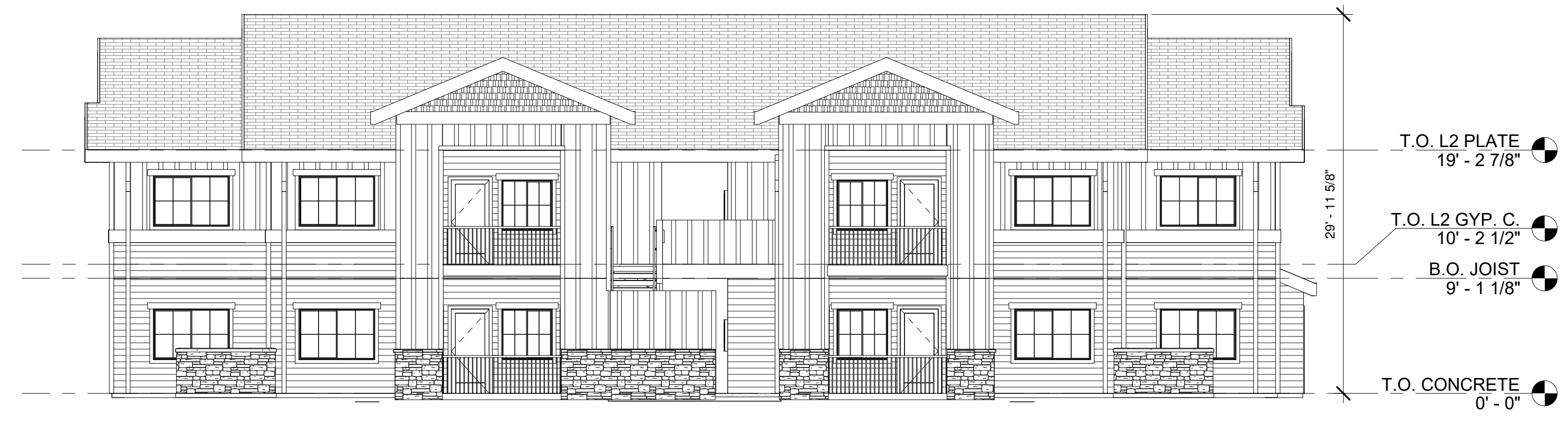
① FRONT ELEVATION - BLDG. TYPE B 1/8" = 1'-0"
