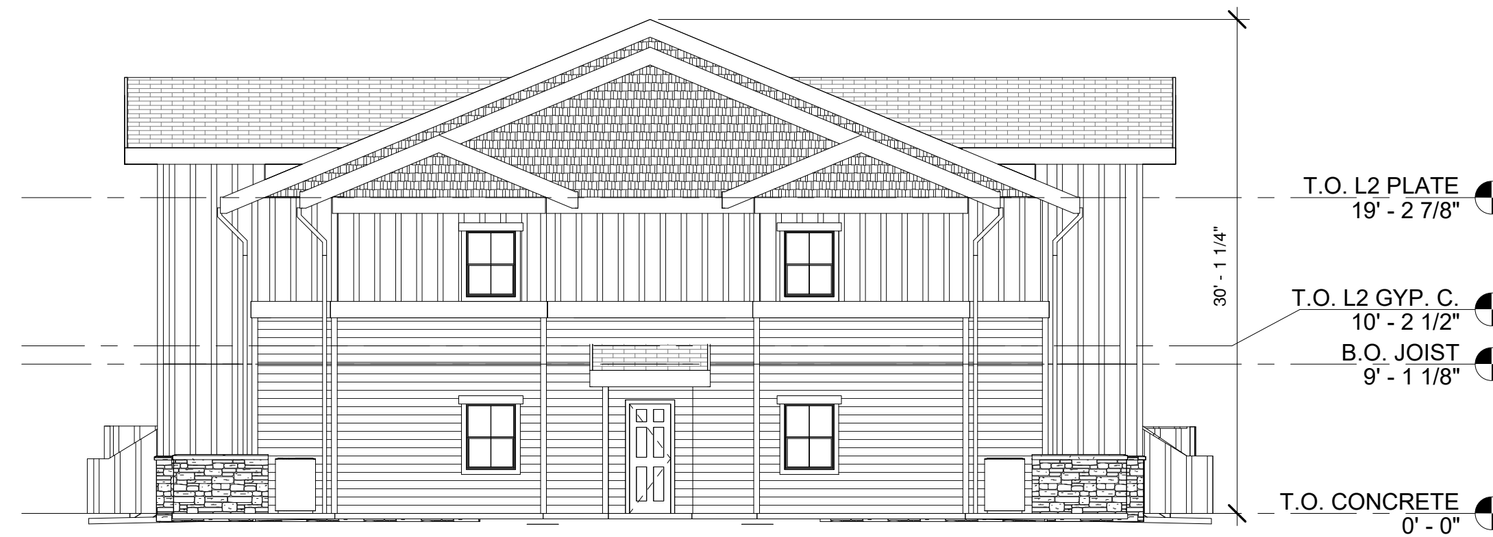
3 RIGHT ELEVATION - BLDG. TYPE A 1/8" = 1'-0"
